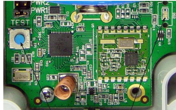
Test Mode Switch      Test Mode LED
